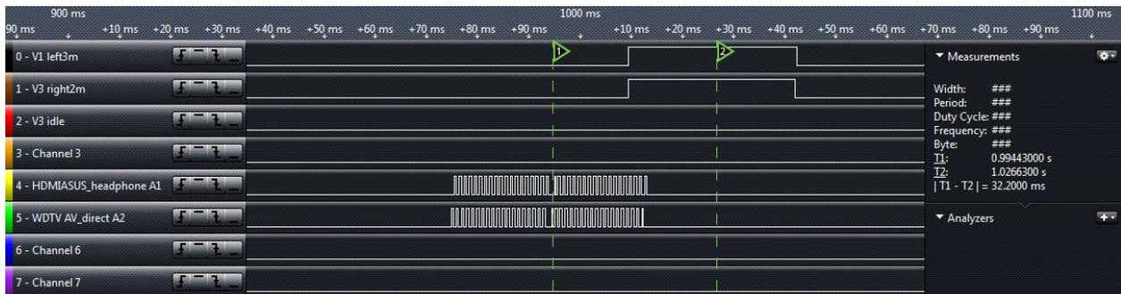
Zooming to the front edge of video pulses makes visible even very small timing differences. In this example  $T1 - T2 = 10$  us, i.e. 0.01 ms.
