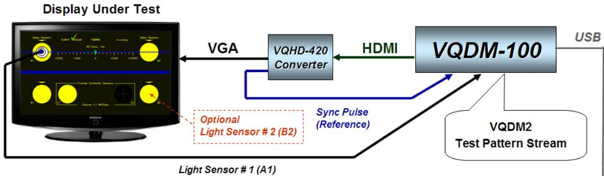
VQDM methodology also allows measurement of display latency spatial (horizontal and vertical) profile by comparison of:
