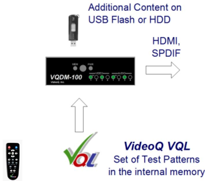
VQDM TPG module is equipped with digital HDMI and SPDIF outputs plus baseband analog YPrPb and NTSC/PAL CVBS video outputs as well as analog L-R audio outputs.
