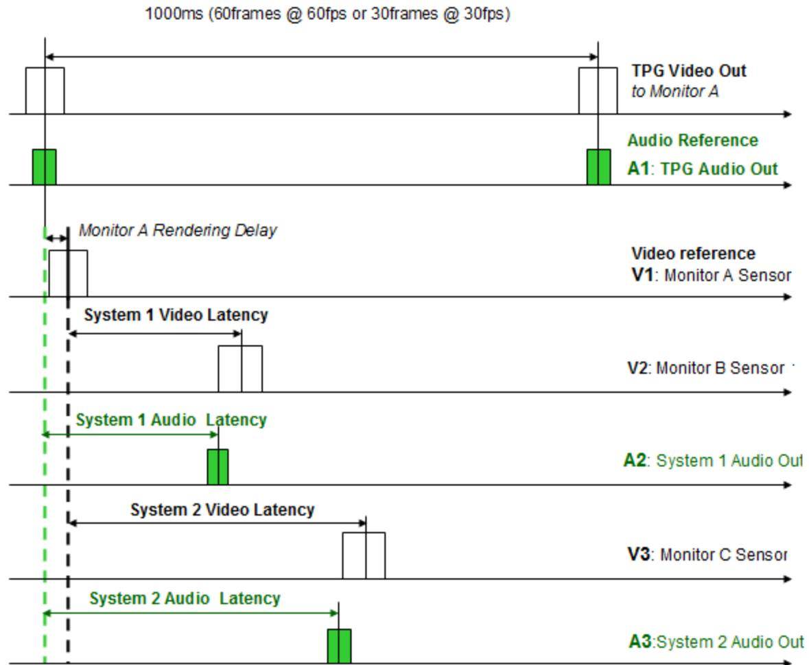
On this diagram two *Systems* are tested in one VQDM *Test Session*.
