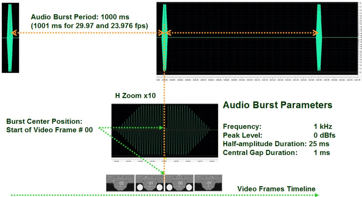
The audio burst central gap can be used as a precise time stamp for very accurate audio timing measurements whilst using waveform monitor or AV editing software.
