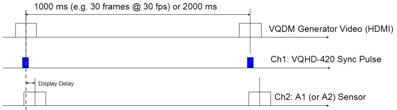
**Display Latency = Light Sensor Pulse Time Position – Reference Sync Pulse Position**
