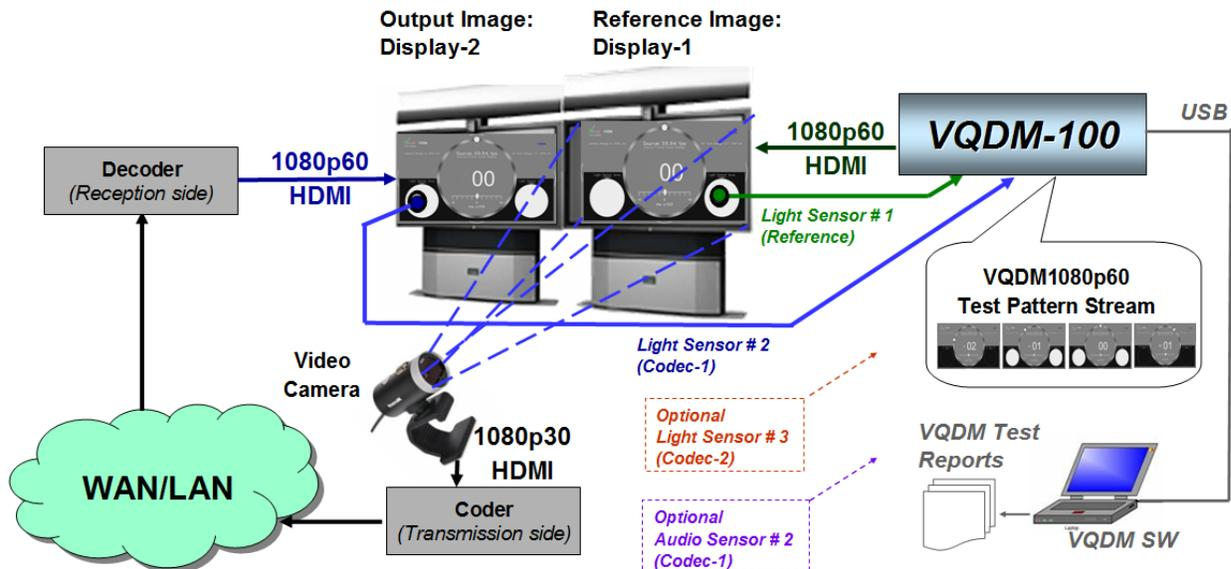
In this example glass-to-glass latency measurement covers complete system:
