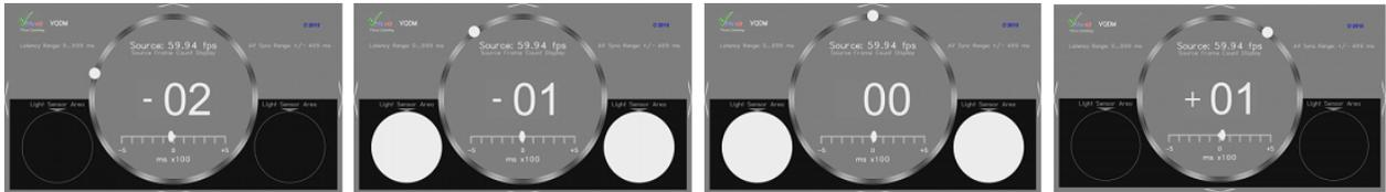
Two large **Light Sensor Areas** on the Test Pattern are flashing white *every second* for the duration of *two video frames*.
